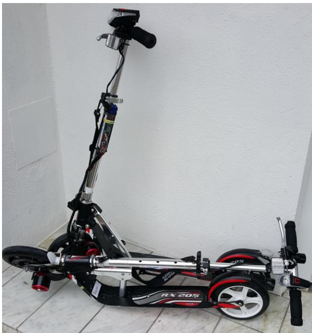
Figure 1. Electrified folding scooters (ca. 250€/1,3kg additional cost/weight).
