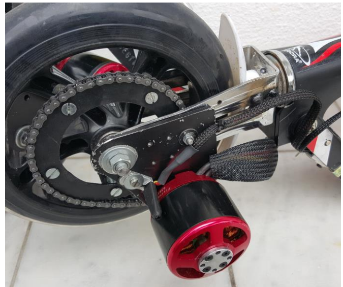
Figure 2. Electrified folding scooter front wheel add-on kit.
