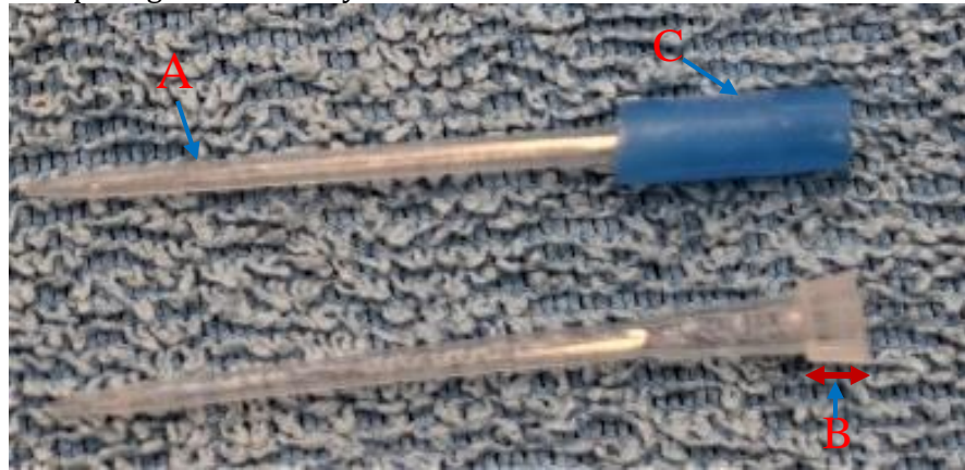
Figure 1. Supplied nozzle (A) with a bottom to be cut off (B) and replaced by nylon pipe (C).
