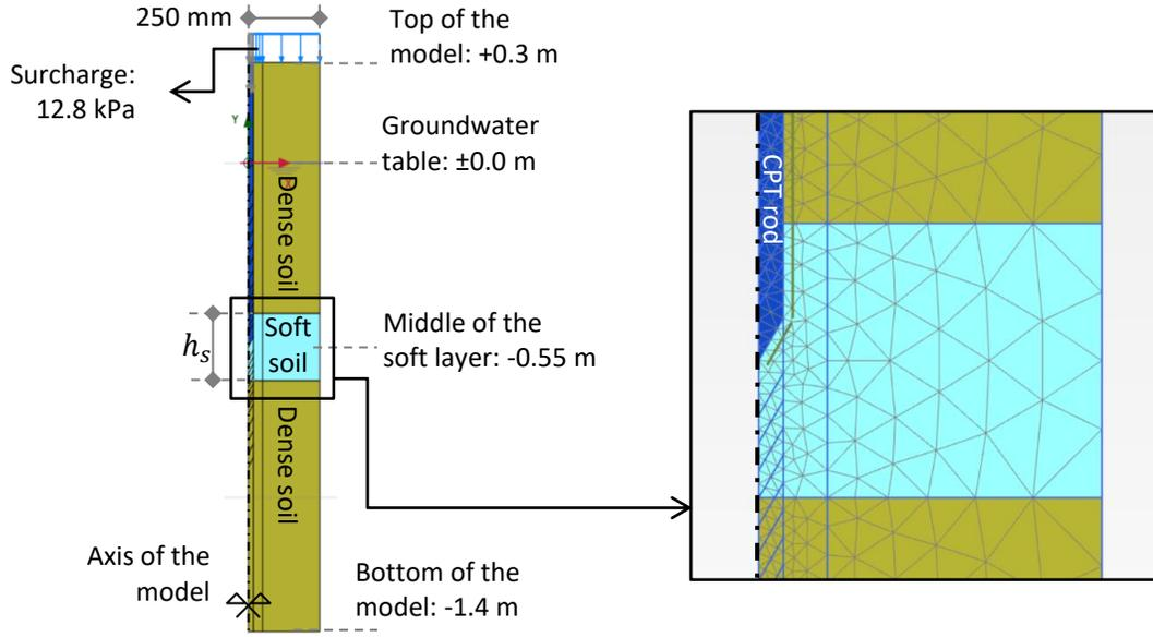
Figure 1. Geometry of the modelled conditions.
