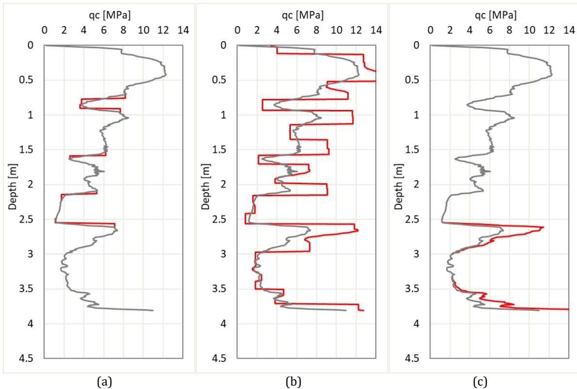
Figure 9. Thin layer correction according to (a) this study, (b) Boulanger and DeJong and (c) de Greef and Lengkeek
