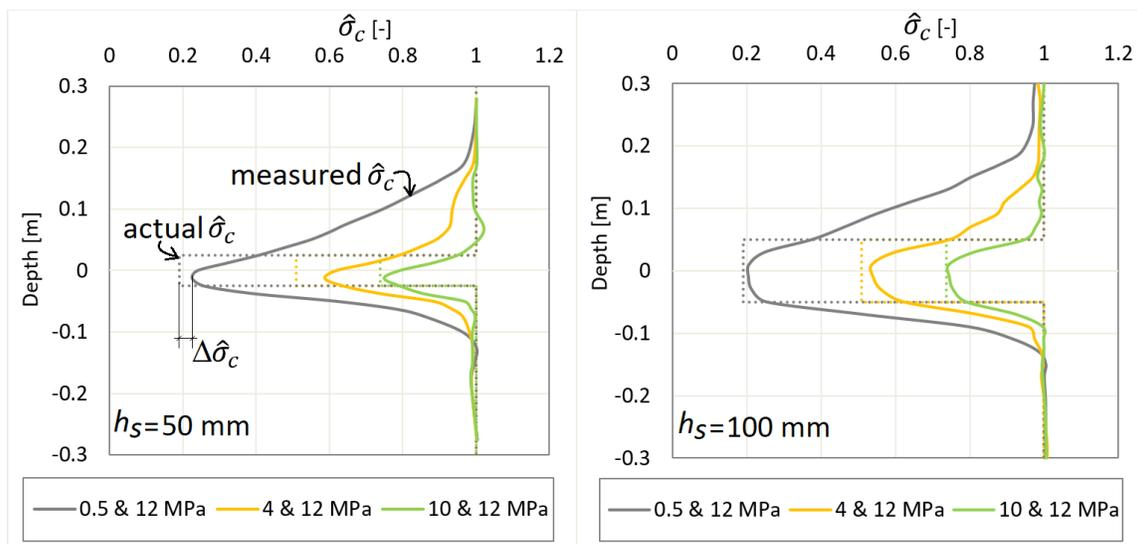
Figure 5. Measured and actual  $\hat{\sigma}_c$  for  $h_s=50$  and 100 mm ( $E_s$  and  $E_d$  are given in the legend).
