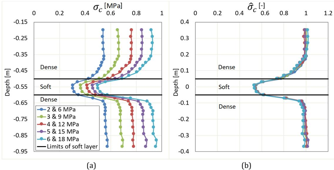
Figure 2. (a)  $\sigma_c$  and (b)  $\hat{\sigma}_c$  for  $h_s=10$  cm and  $R_s=0.333$  ( $E_s$  and  $E_d$  are given in the legend).
