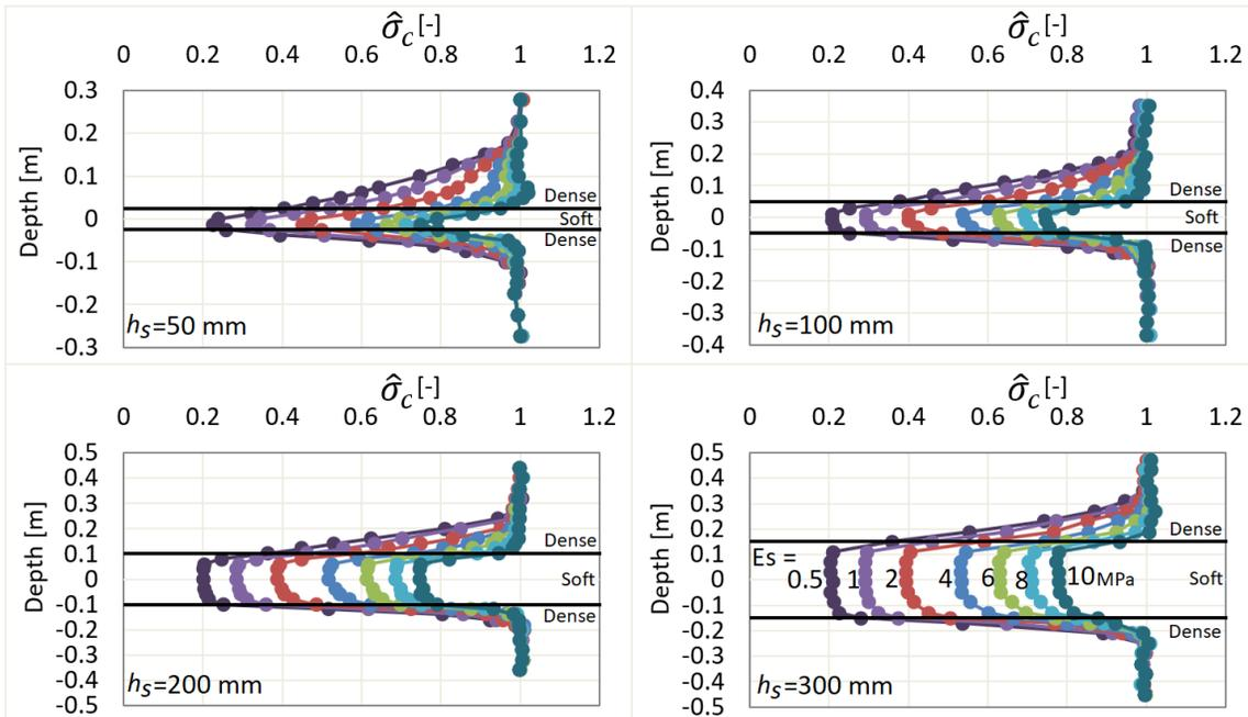
Figure 3.  $\hat{\sigma}_c$  for different soft layer thicknesses ( $h_s$ ).  $E_s=12$  MPa ( $h_s$  and  $E_s$  are given on the graphs).
