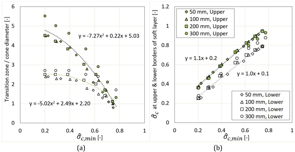
Figure 4. (a) TZ in the upper and lower dense soils divided by  $d_c$ , (b)  $\hat{\sigma}_c$  at upper and lower borders of soil layers, plotted against  $\hat{\sigma}_{c,min}$  ( $h_s$  is given in the legend).
