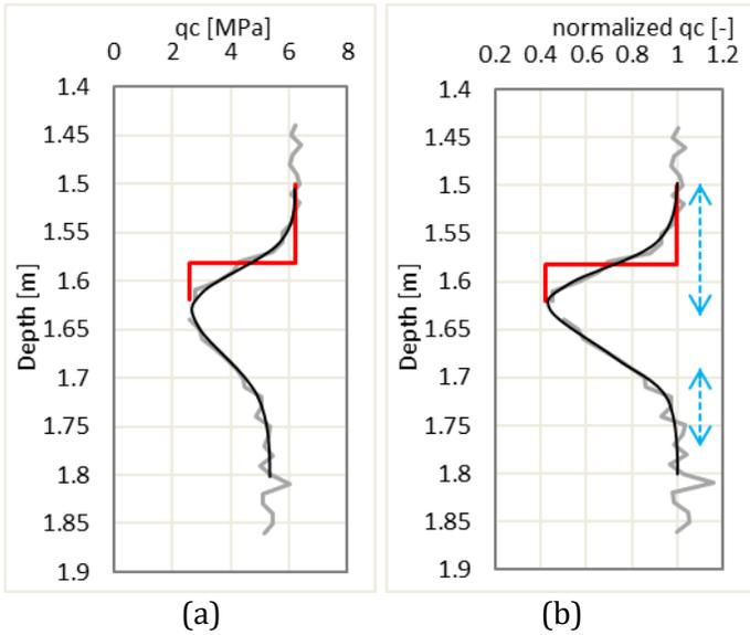
Figure 8. (a) measured and corrected  $q_c$  values, (b) normalized  $q_c$  values
