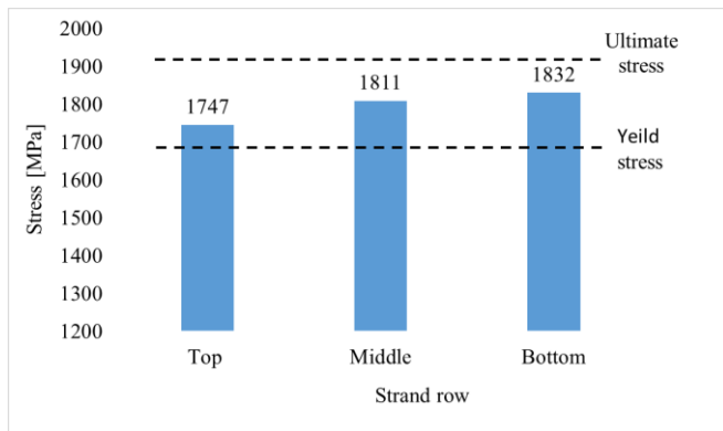
Figure 9. Stresses along the strands of the beam at failure.
