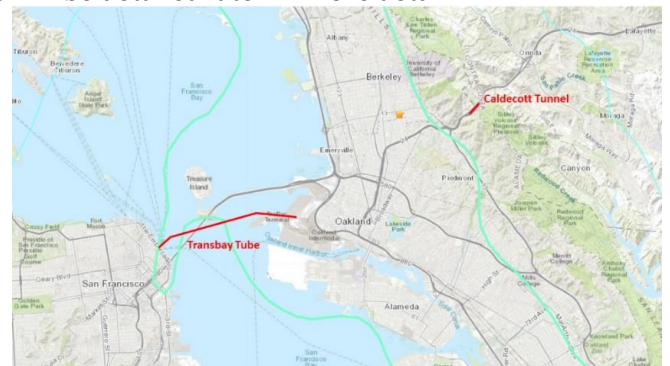
Figure 4. Locations of the epicentre (Berkeley Earthquake of 04 Jan 2018, Mw=4.4, 02:39:37 PST, 37.8552N 122.2568W Depth 12.3 km), indicated by ☆, and the two infrastructures, highlighted in red, with shakemap MMI contours superimposed in green.
