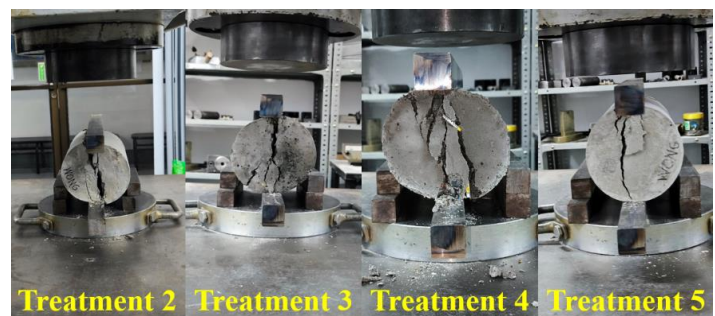
Figure 8. Type 3 failure in tensile test.
