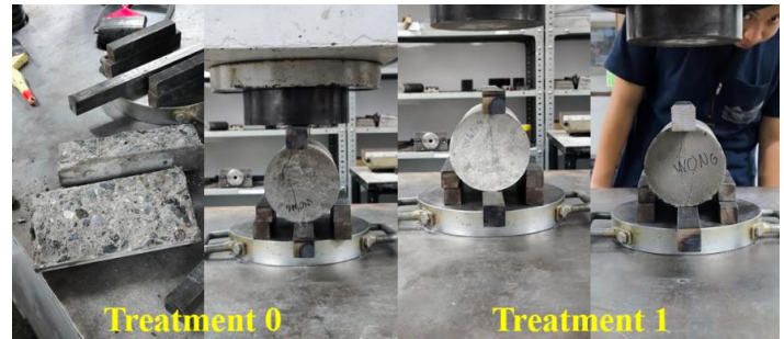
Figure 7. Type 2 and type 1 failure in tensile test (left to right).
