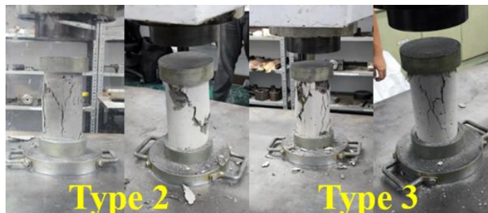
Figure 6. Examples of type 2 and type 3 failures.
