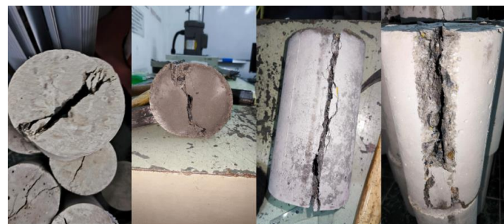
Figure 9. Samples of type 3 failure outside the UTM.
