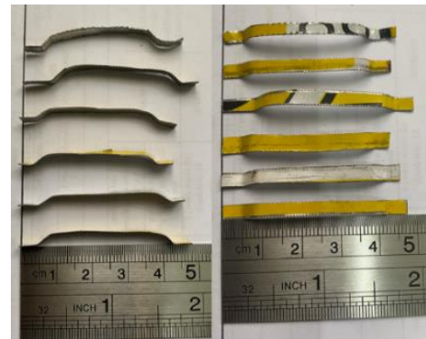
Figure 2. Produced recycled steel can fibers.
