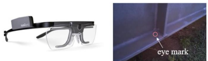
Figure 2. Eye-tracking device used during inspection.
