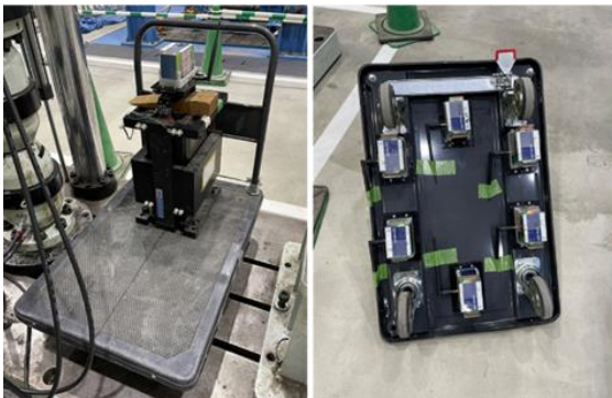
Figure 12. Excitation test of the dolly
