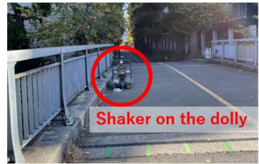
Figure 15. Dolly test on the bridge
